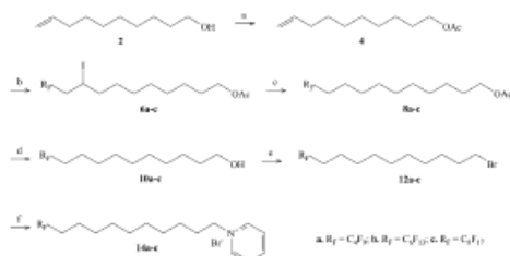
Scheme 2 a. DMAP, AcCl, pyridine, DCM; b. \text{R}_F\text{I} , AIBN, \Delta ; c. HI (55%), Zn, \text{C}_2\text{H}_5\text{OH} , \Delta ; d. \text{CH}_3\text{OH} , KOH, \Delta ; e. \text{PPh}_3 , \text{Br}_2 , DCM, ambient temperature; f. pyridine, \Delta .
