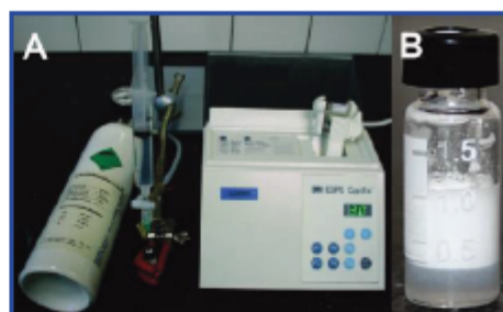
Figure 1. Equipment for preparation of MB: (A) capsule mixing device (3M ESPE CapMix) and the small bomb with sulfur hexafluoride (SF 6 ) linked with three-way valve and syringe for filling vials. (B) Sealed vial with dispersion of MB under a SF 6 atmosphere.
