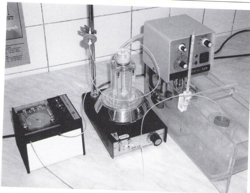
FIG. 3. Entire system for the preparation of liposomes by the proliposome-liposome method.
